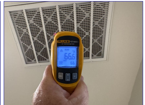
The furnace and AC system was operated using the wall mounted thermostat. The furnace and AC system were run for ten minutes and the air was tested with an infrared thermal meter before and after running the systems, showing a temperature change of more than ten degrees at the air register in the rooms of the home. The test shows the systems were functional at time of inspection.
